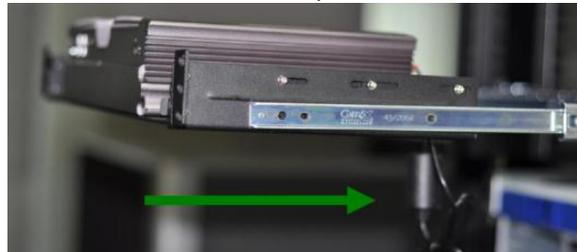
3. Holding the unit with its front facing you, lift the supporting frame and carefully insert the unit by sliding the inner rails into the rack's rail.
