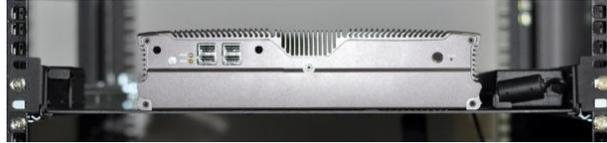
**(Option 2) Position the server rack rails alongside the unit.**
